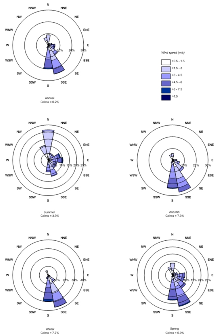
Figure 3: Olkaria wind roses derived from Calmet Model at 10m above ground level
