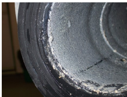
Figure 6: Biofilm growth on first section of 100 mm dia. pipe
