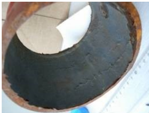
Figure 8: Pipe removed from the reinjection line and covered with black deposits
