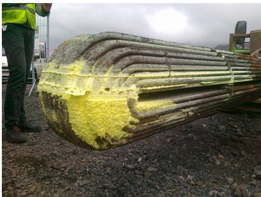
Figure 4. Heating element from the bottom distillation column in the pilot gas separation station in Hellisheiði power plant, Iceland. The yellow colour is elemental sulphur. Rust colour on the cooling element on the right of the picture is where drops of liquid H_2S /water mixture fall on the heating element.
