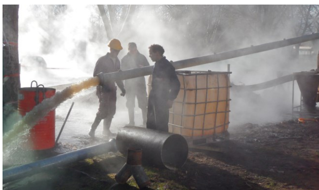
Figure 5: Air flow production test, well CC3 with geothermal fluid at 74°C, Chaves geothermal field (January 2014).
