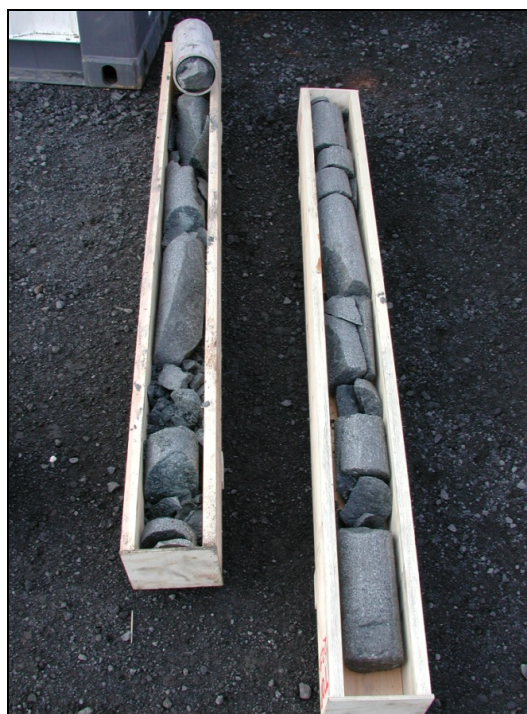
Figure 8: The core cut into a dolerite intrusion with high angle actinolite veinsf that are quite visible in the box to the left. The top of the core is in the box to the right - bottom right corner of the image, looking downwards. The boxes are 1.6 m long and the aluminum liner is still around the bottom of the core
