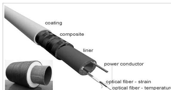
Figure 9: Composite tubing developed by Delft University, WEP and Airborne and proposed by Acquit, to be used as an innovative alternative drilling/well option for steel tubing
