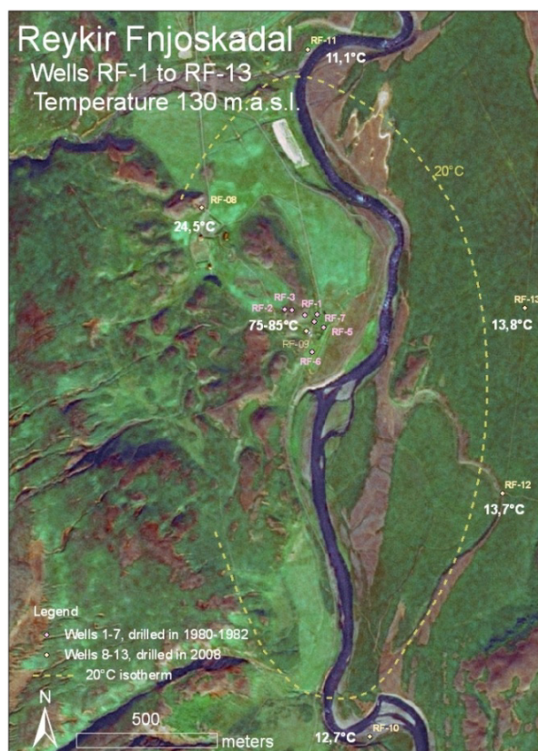
Figure 5: Measured temperature 130 m.a.s. in boreholes in Reykir and a 20°C isotherm.
