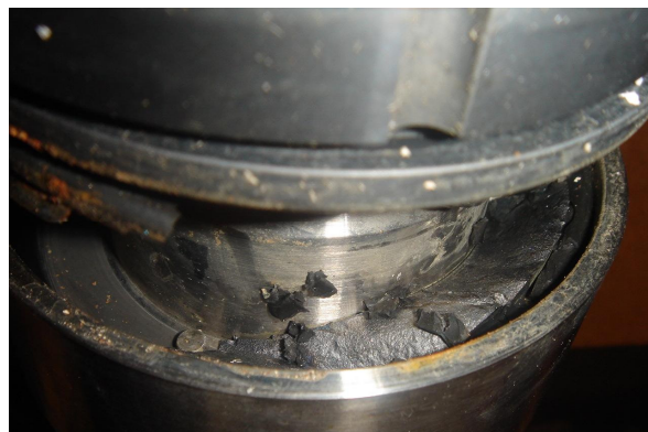
Figure 7: Mechanical seal ceramic failure.
