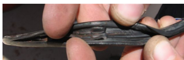
Figure 5: Seal failure due to explosive decompression.
