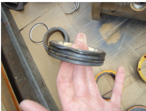
Figure 6: Seal failure due to extrusion.
