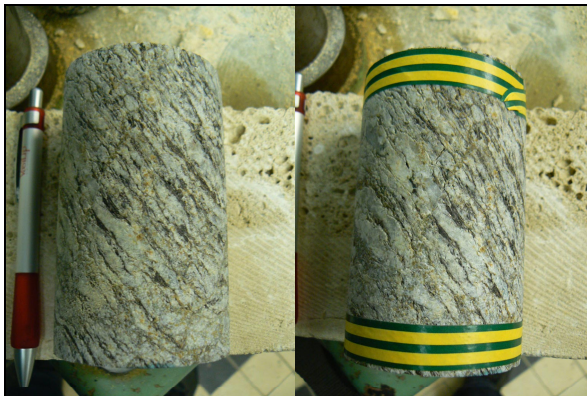
Figure 3: The investigated sample before and after the cyclic loading test
