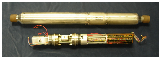
Figure 2: Sandia-designed seismic tool commercialized with OYO.
