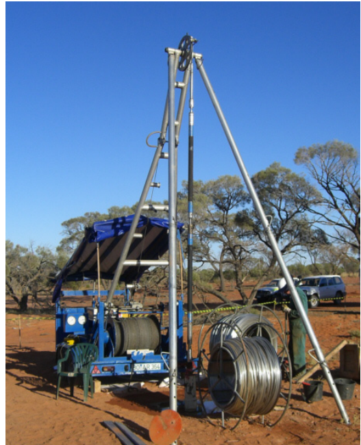
Figure 4: Hydrofrac Equipment MeSy MKW-2000. The straddle packer tool is shown being prepared for running into Blanche 1
