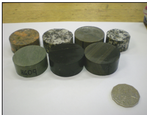
Figure 5: Selection of samples cut to ~2cm in length and with both ends polished.
