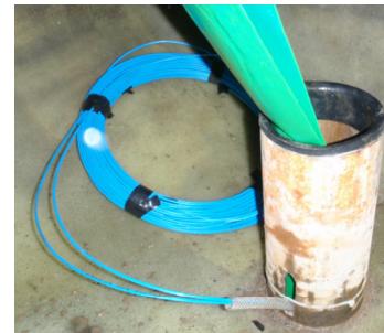
Figure 5. Energy capsule already installed and before water filling. The external fiber cable is taken out through a trace opened in the steel casing
