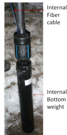
Figure 6. Central pipe, internal bottom weight and fiber cable
