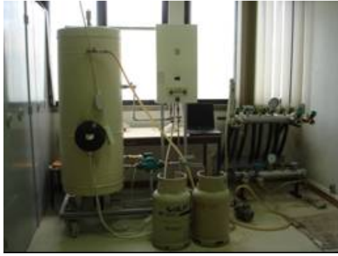
Figure 10: Experimental device to perform the thermal response test
