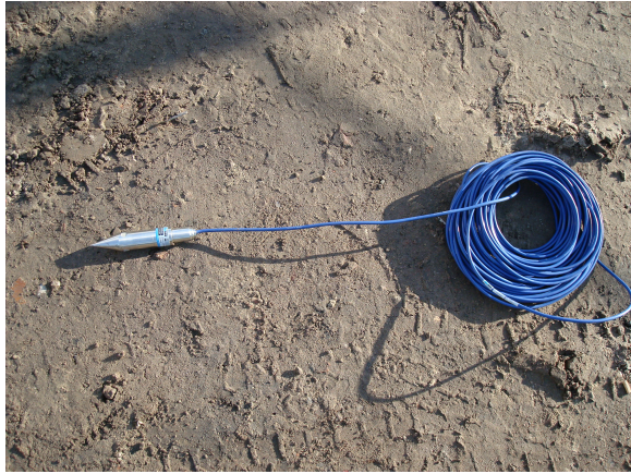
Figure 12: Penetration cone with installed temperature sensor.
