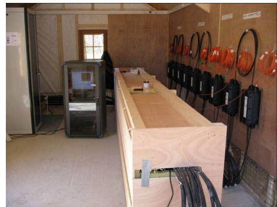
Figure 6: Measurement optical fibers and signal analysis implemented in the second hut
