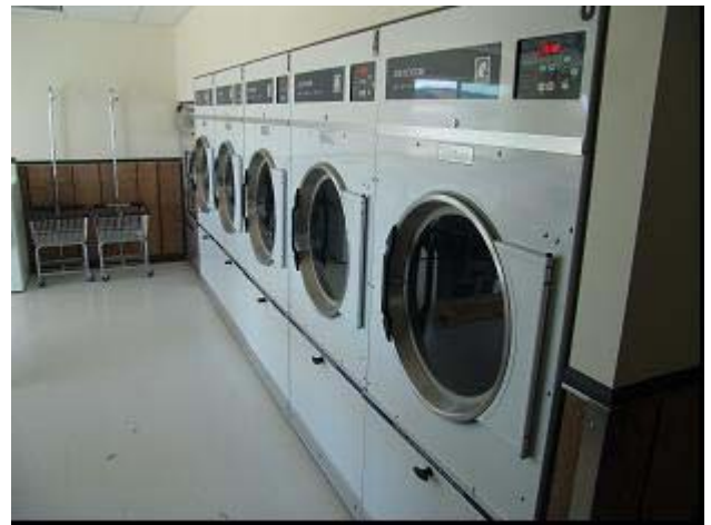
Figure 6: Retrofitted 55 lb. Industrial Dryers
