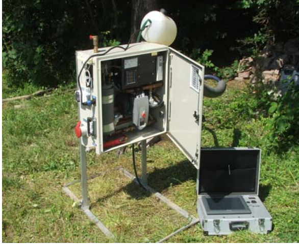
Figure 2: Device of thermal response tests.
