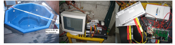
Figure 5: The experiment layout and arrangement of thermocouples for data gathering process.
