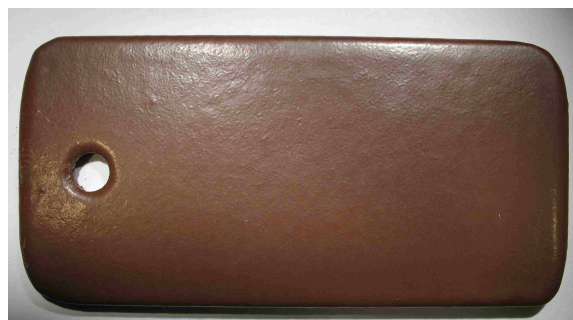
Figure 7: Photograph of the specimen coated with Sakaphen synthetic coating after test EGS_02. Test conditions: 200 °C, 0.5 bar CO 2 , pH 4.6-5, brine (see Table 3)
