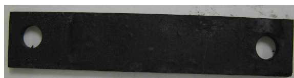
Figure 14: Photograph of the non-coated TU42BT steel specimen after test EGS_03. Test conditions: 200 °C, 0.5 bar CO 2 , pH 4.6-5, brine (see Table 3), 10 ppm Mexel inhibitor
