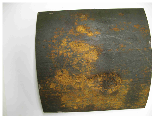
Figure 26: Photograph of the corroded part of the pack-off assembly of casing in the injection well GPK3 suspected for microbiological corrosion
