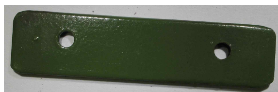
Figure 9: Photograph of the specimen coated with the green Teflon coating after test EGS_02. conditions: 200 °C, 0.5 bar CO 2 , pH 4.6-5, brine (see Table 3)
