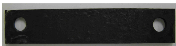
Figure 15: Photograph of the non-coated P110 steel specimen after test EGS_03. Test conditions: 200 °C, 0.5 bar CO 2 , pH 4.6-5, brine (see Table 3), 10 ppm Mexel inhibitor
