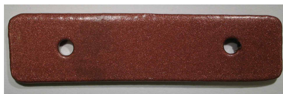
Figure 8: Photograph of the specimen coated with the red Teflon coating after test EGS_02. Test conditions: 200 °C, 0.5 bar CO 2 , pH 4.6-5, brine (see Table 3)
