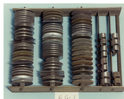
b. Pictures of coupons on a loaded rack for exposure inside Vessel 6, Cold Condensate.
