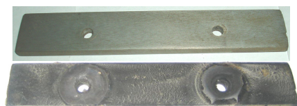
Figure 3: Metal coupon before (above) and after (below) the field testing experiment at the third pipe section, with acid-treated geothermal brine at \sim 120^{\circ}\text{C}
