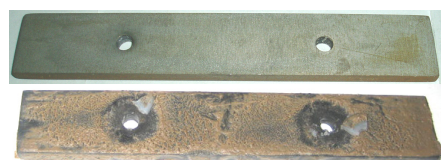
Figure 4: Metal coupon before (above) and after (below) the field testing experiment at the fourth pipe section, with acid-treated and organic chemical inhibitor injected geothermal brine at \sim 120^{\circ}\text{C}
