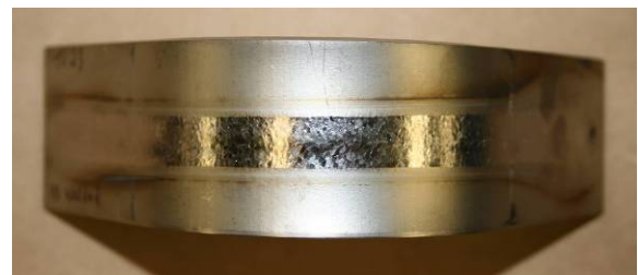
Figure 3: Example of Welded Material After Forming, Gr23.
