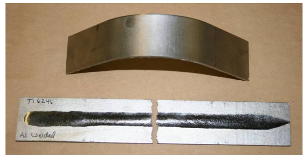
Figure 2: Ti 6246 Forming Results, Base and Welded Material.
