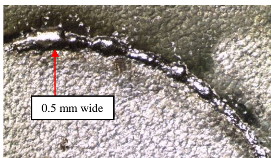
Figure 4: Crevice Corrosion of Alloy 625.
