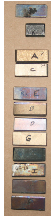
Figure 1: Coupon Samples Showing Their Colors After Condition 2 Testing.
