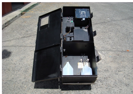
Figure 5a: Continuous flow analyzer from Rosemount Analytical Inc. Photo by P. Moya.
