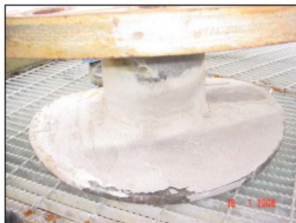
Figure 10: Deposit on separator bottom.
