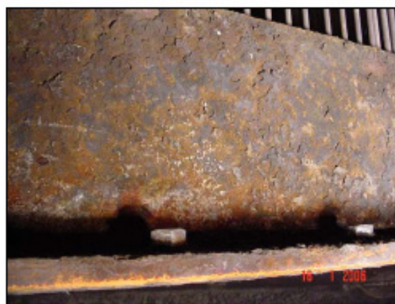
Figure 8: Corrosion on demister elements holder damaged some demister elements.
