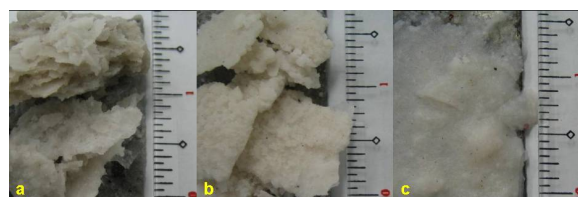
Figure 3: Characteristics of deposits at the open pipe using A ppm F3680 a) layers of thin but moderately hard; b) granular and compact; c) very soft and porous
