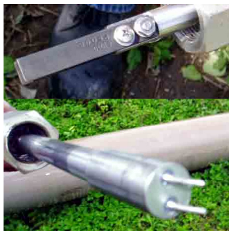
Figure 3: Corrosion rates were monitored using an LPR corrosometer (bottom) and corrosion coupons (top)
