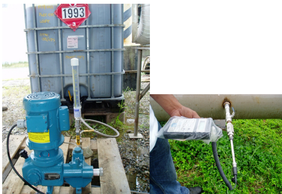
Figure 2: Test set-up consisting of a dosing pump, calibration column and a tank for the corrosion inhibitor (left photo). Corrosion monitoring from an LPR test probe was inserted along the condensate line (right photo)
