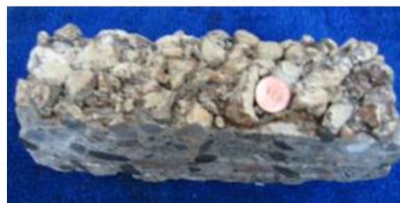
Figure 8: Rock aggregates protruding out of the corroded concrete surface.
