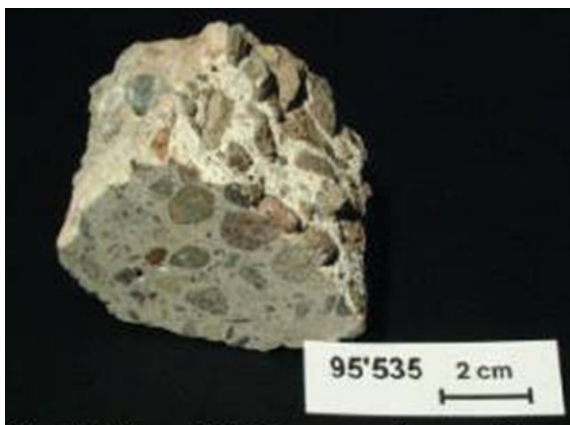
Figure 1: Rock Muffler sample shows removal of cementitious matrix, leaving aggregates exposed.
