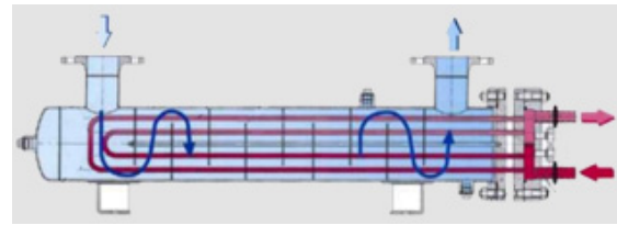
Figure 3. Schematic of shell and tube heat exchanger, Source; www.mdtofis.com
