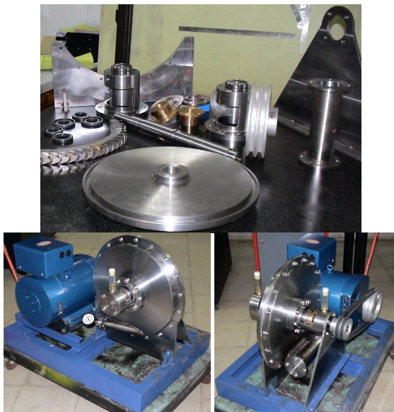
Figure 14. Photo of parts and assembly of 2 kW n-pentane turbine
