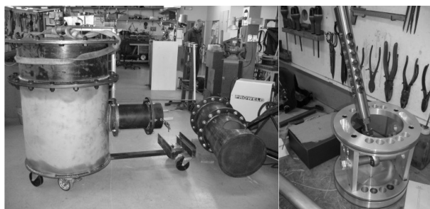
Figure 4: Photographs of the initial research engine/electric generator design currently being fabricated. The main pressure chambers are shown on the left, and the power piston is shown on the right.
