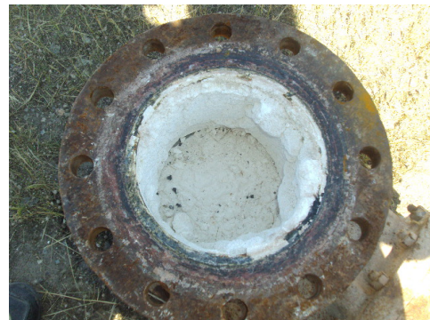
Figure 1: Calcite scaling in the wellbore
