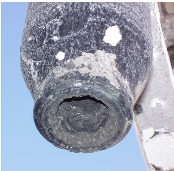
Figure 2: Silica scaling in a brine injection pipe after one year operation.
