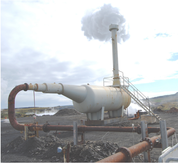
Figure 9: The horizontal separator/silencer for well testing
