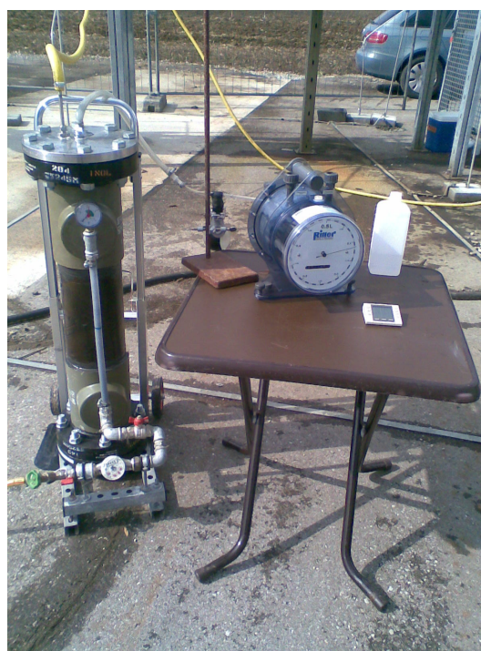
Figure 3: Set-up of measuring instruments for gas sampling
