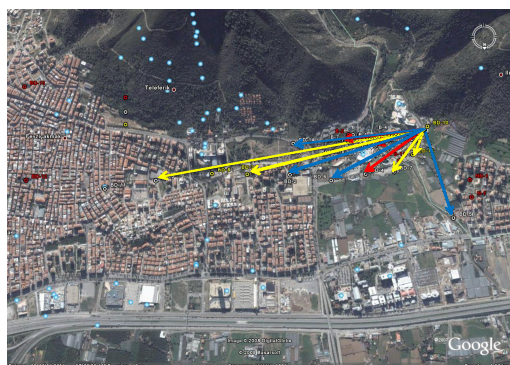
Figure 5: NaCl flow direction based on mean arrival times in production wells
