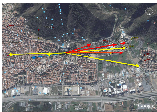
Figure 6: Rhodamine B flow direction based on mean arrival times in production wells
