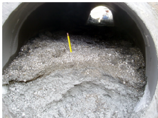
Figure 4. Solids discharged by the well and collected from the solids trap consists mostly of formation rocks with small amounts of corrosion products and silica scales. Silica forms a thin layer around the solids which binds the solids together. The petrology of the rocks gave a clue to the source production well.
