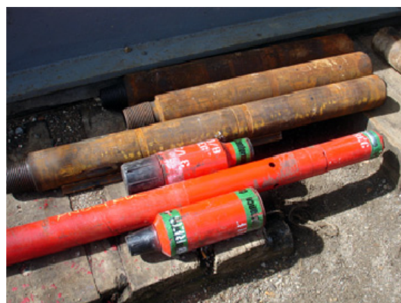
Figure 11. The venturi jet assembly was used during the last workover in KN1RD to remove the solids fill at the bottom of the well which cannot be circulated out by the rig.
