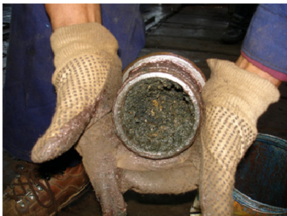
Figure 12. Sand sized rocks collected by the venturi jet from KN1RD. Although the tool was successful in capturing a large amount of solids, the limited volume of the tool requires multiple run-ins which were considered impractical.
