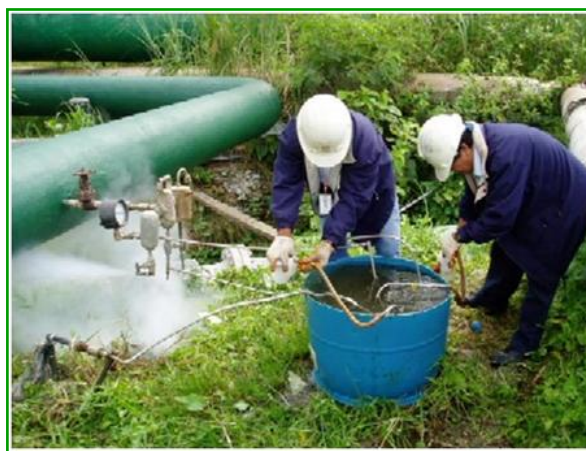
Figure 4: Sampling set-up adapted for tritium collection in highly two-phase wells.
