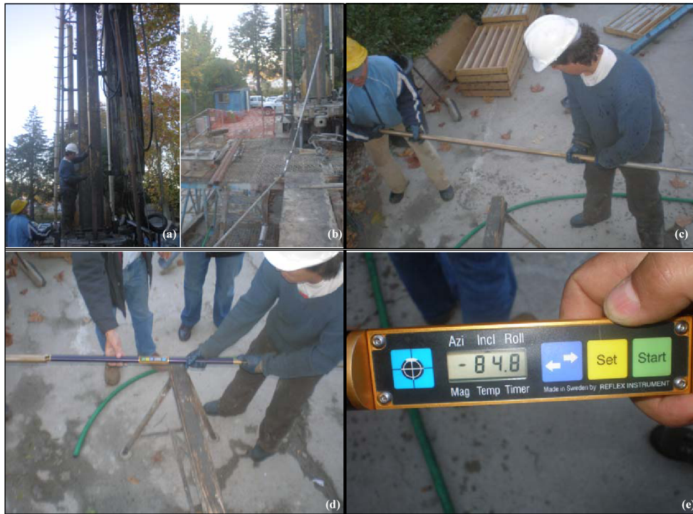
Figure 8: Images of the spatial probing positioning measurements performed with a “Reflex Instruments- EZ-SHOT” device in US1, Unhais da Serra.
