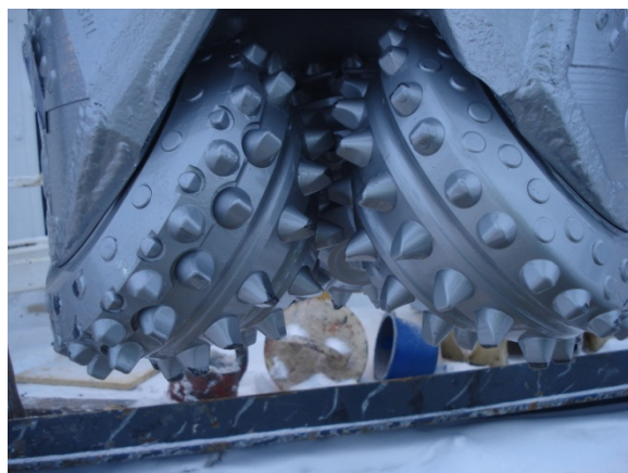
Figure 7. New roller cone bit.
