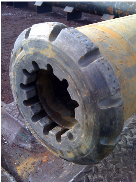
Figure 10. The Core bit after the coring attempt.
