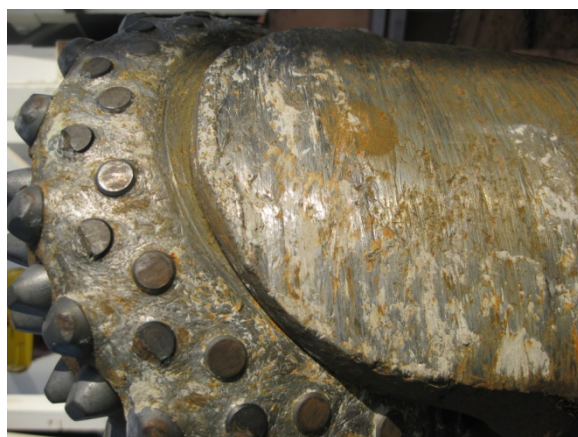
Figure 8. Worn roller cone bit.
