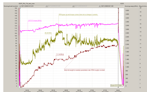
Figure 8: Smoothed Drilling Parameters recorded during the Coring Run (yellow: RPM. Blue: WOB, Dark purple; flush, Light Purple: penetration).
