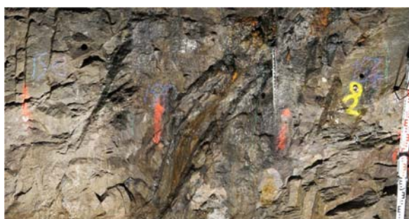
Figure 4: Snapshot by ISIS of the test site in the training and research mine of the TU Bergakademie Freiberg. The red lines show the position of surrounded geophones.
