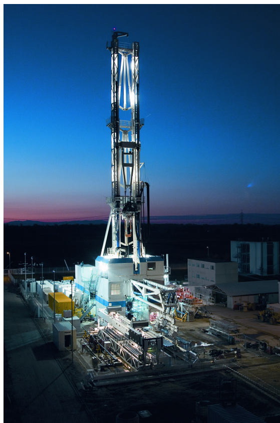
Figure 1: Night view of InnovaRig at the Herrenknecht manufacturing plant in Germany, occupying a 30 x 80 m drill pad and the 50 m high illuminated mast standing ready to receive drill-pipe from the automatic pipe-handler loading doubles from the pipe-rack to catwalk.
