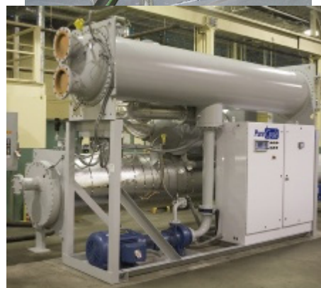
Fig 3. 2 photos of Binary Geothermal units of 50KVA and 280KVA
