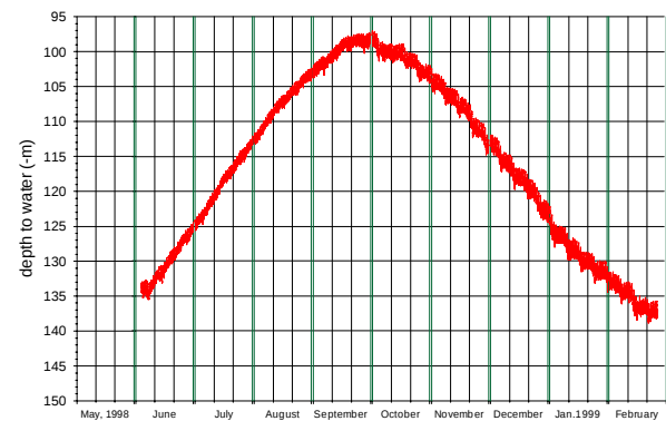
Figure 5: The change of the piezometric head from June, 1998 to February, 1999.
