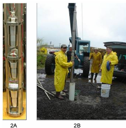
Figure 2: (2A) = Inside of the 3-component borehole seismometer. Top geophone is vertical; middle and bottom geophones are horizontal and orthogonal. Geophones are the small cylinders; the large conical shapes are gimbaled counterweights to control for borehole tilt and contribute to damping. (2B) = Installation of a seismometer into a standard diameter HQ borehole. Top half of the instrument is a tiltmeter.
