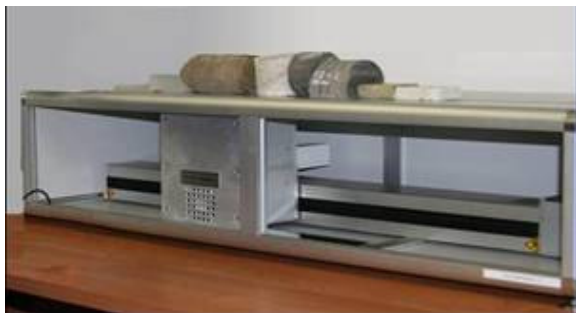
Figure 2: Optical scanning instrument for rock thermal property measurements on full cores.
