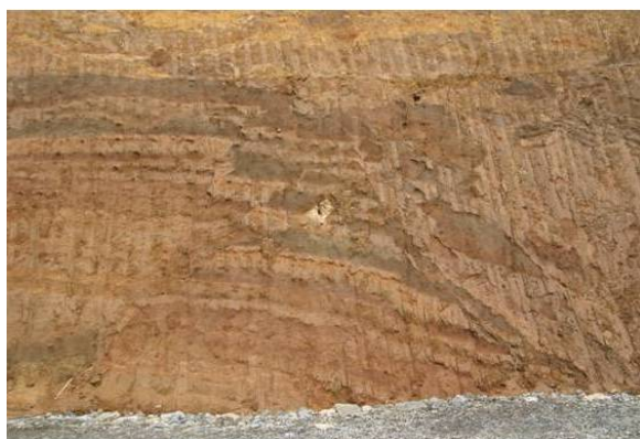
Figure 7. Subsidiary NE-trending fault and breccia zone on the W side of the Gareok fault. Note disrupted beds of Upper Brown tuff on the lower bench and Orange and Upper Brown tuff on the upper bench of the road cut.
