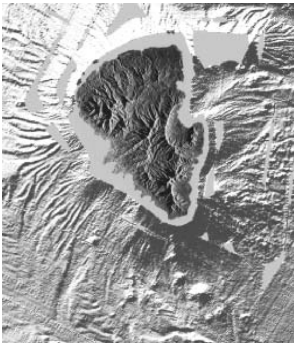
Figure 4: Topography of Lihir Island and bathymetry of the surrounding sea floor (from Herzig et al 1994), showing a debris flow extending offshore to the northeast from Luise Harbour. This figure covers an area about 30 km by 40 km; Lihir Island is 22 km long
