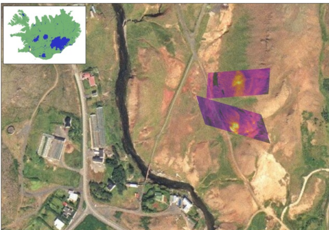
Figure 3. Obliquely georeferenced thermal images in the same area.
