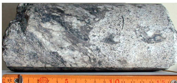
Figure 8: A spot core sample from 2,842-2,844 m depth of WD-1a, the Kakkonda geothermal field in Sengan, Tohoku.
